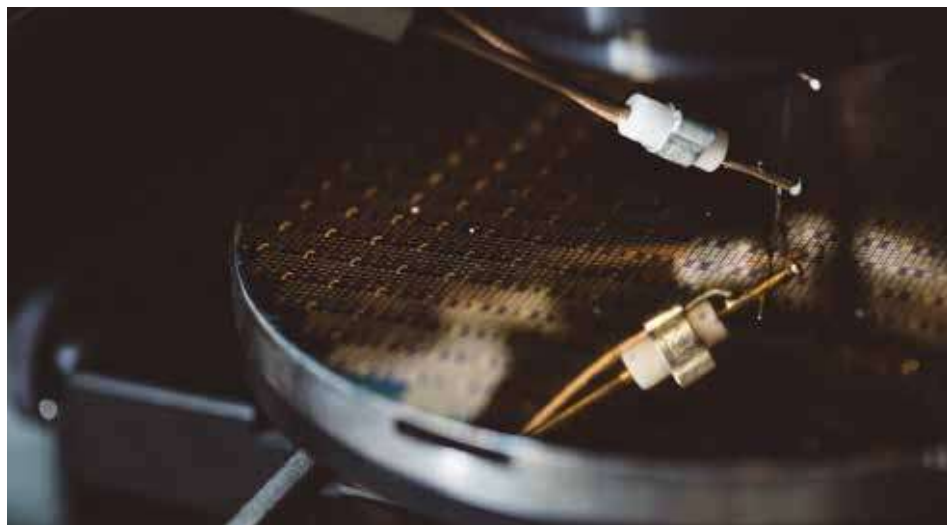
A 150mm wafer of GaN microLEDs under test via wafer probing
